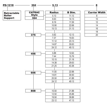
For radii not shown and for multiple carrier widths, consult factory.
