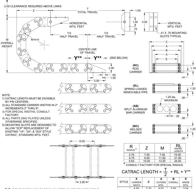
\*\* IF THE STATIONARY FOOT IS MOUNTED ON EITHER SIDE OF THE CENTER LINE OF TRAVEL, THE DISTANCE (Y) BETWEEN CENTER LINE AND STATIONARY FOOT MUST BE ADDED TO CATRAC LENGTH.
