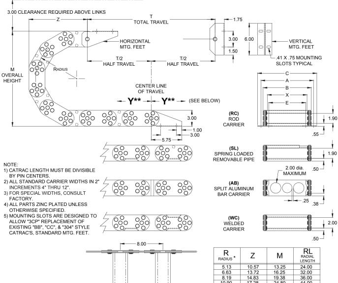
\*\* IF THE STATIONARY FOOT IS MOUNTED ON EITHER SIDE OF THE CENTER LINE OF TRAVEL, THE DISTANCE (Y) BETWEEN CENTER LINE AND STATIONARY FOOT MUST BE ADDED TO CATRAC LENGTH.
